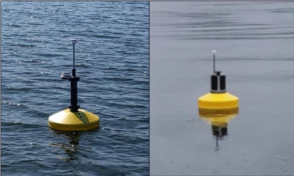
*Figure 2. MarineLabs CoastScout buoys deployed at the sites. (left) older generation, (right) current generation CoastScout.*
