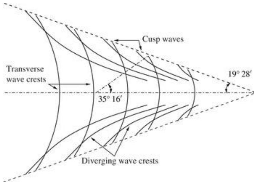
Figure 4. Vessel wake diagram showing divergent and transverse waves with wave cusp line angle at  $35^\circ$  from direction of vessel motion [2].
