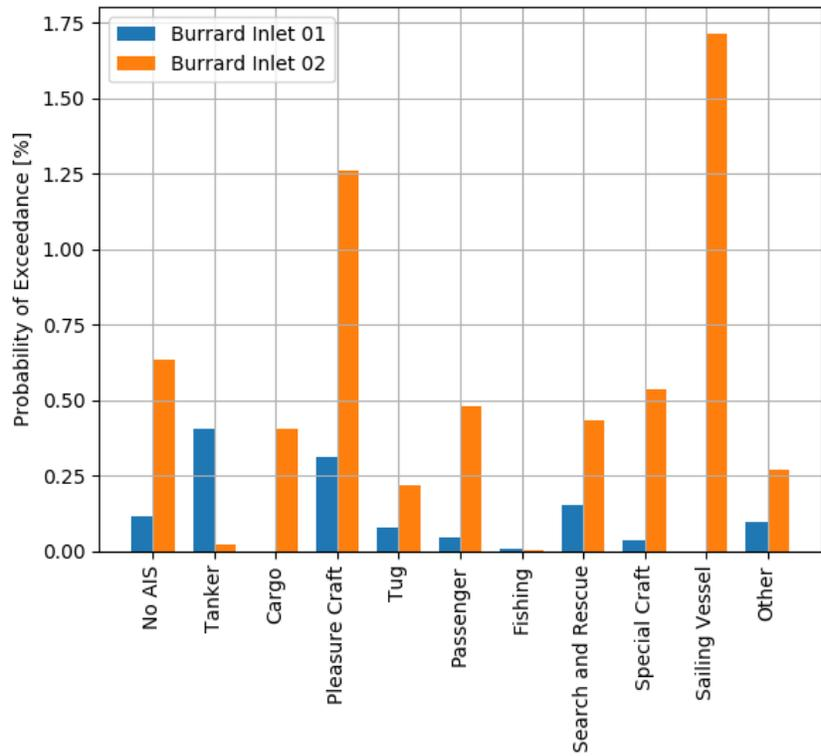
Figure 18: Conditional probability of wave power exceeding 200 W/m for vessel wakes at Burrard 1 and 2.
