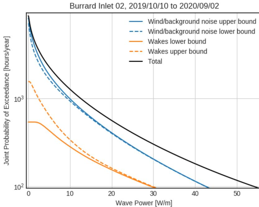
Figure 9: Burrard 2 probability of exceedance distributions for wakes and wind/background noise. The wake upper bound and wind/background noise lower bound are estimated from the automatic wake detection uncertainty analysis. The total probability distribution for all waves is also included. Top: full range of distributions. Bottom: zoomed to illustrate the uncertainty bounds at low power levels.
