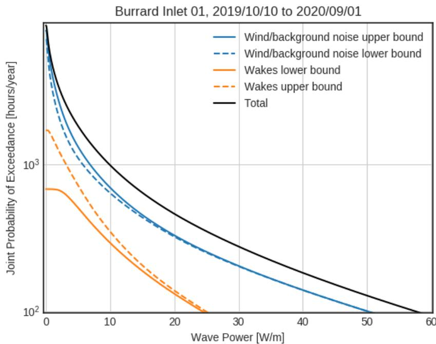
Figure 8: Burrard 1 probability of exceedance distributions for wakes and wind/background noise. The wake upper bound and wind/background noise lower bound are estimated from the automatic wake detection uncertainty analysis. The total probability distribution for all waves is also included. Top: full range of distributions. Bottom: zoomed to illustrate the uncertainty bounds at low power levels.
