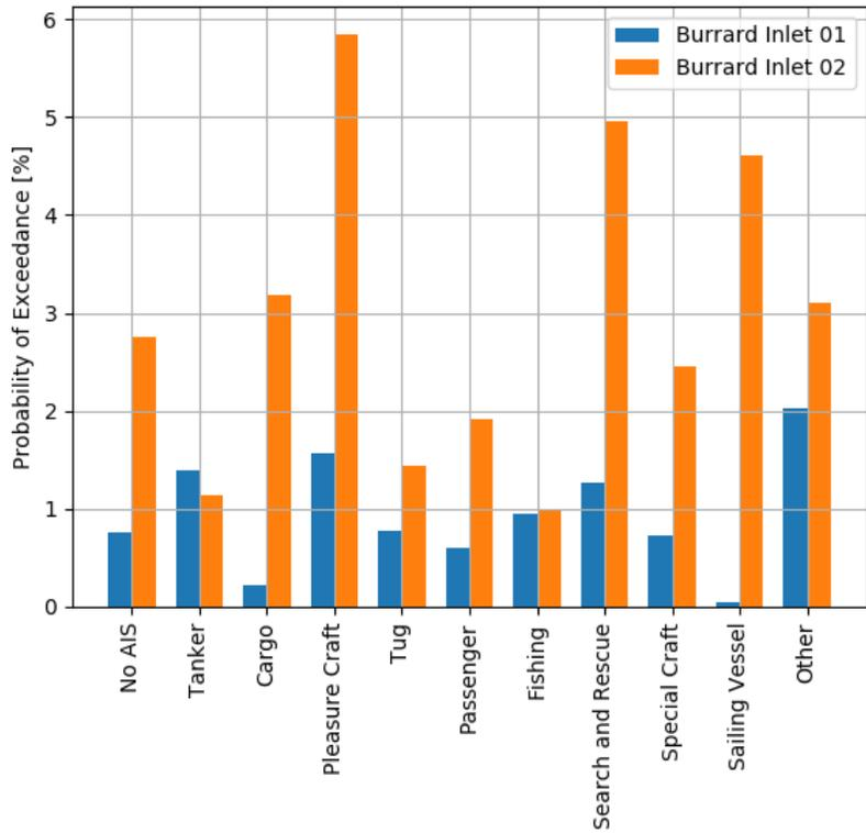
Figure 17: Conditional probability of wave power exceeding 100 W/m for vessel wakes at Burrard 1 and 2.
