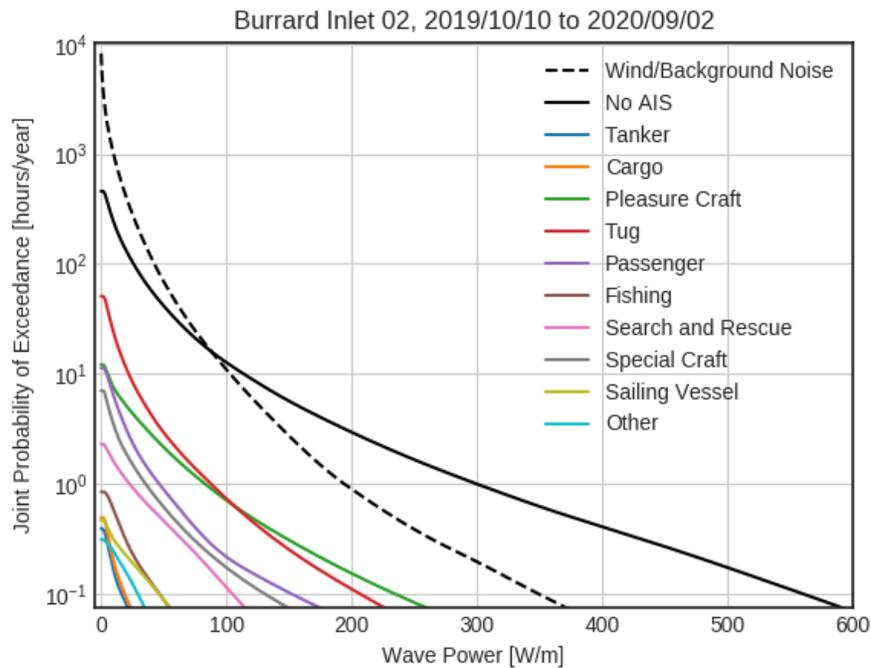
Figure 13: Burrard 2 wave power probability of exceedance distributions based on AIS vessel type.
