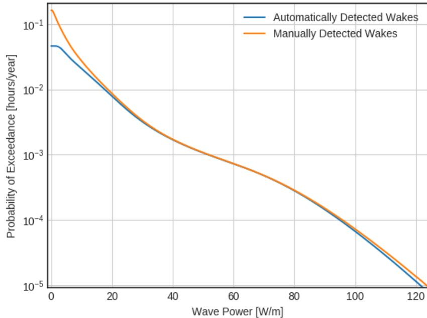
Figure 7: Wave power probability of exceedance distributions using the time intervals of automatically and manually detected wake events.
