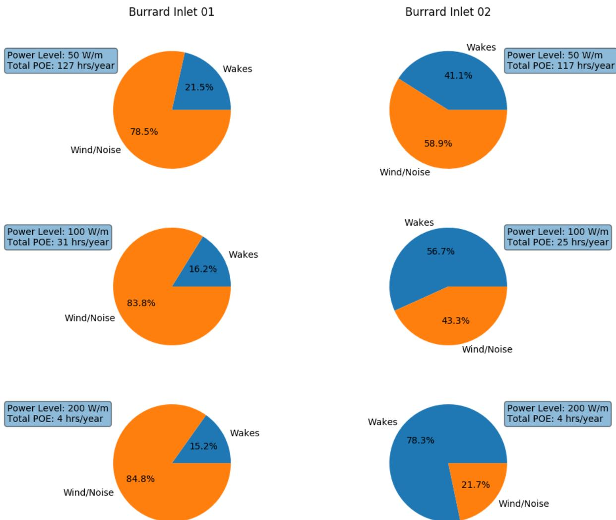
Figure 10: Fractions of the total probability of exceedance distributions for Burrard 1 and 2 that are attributed to wakes and wind/background noise. The three power levels for which the probabilities of exceedance are calculated are 50, 100 and 200 W/m.
