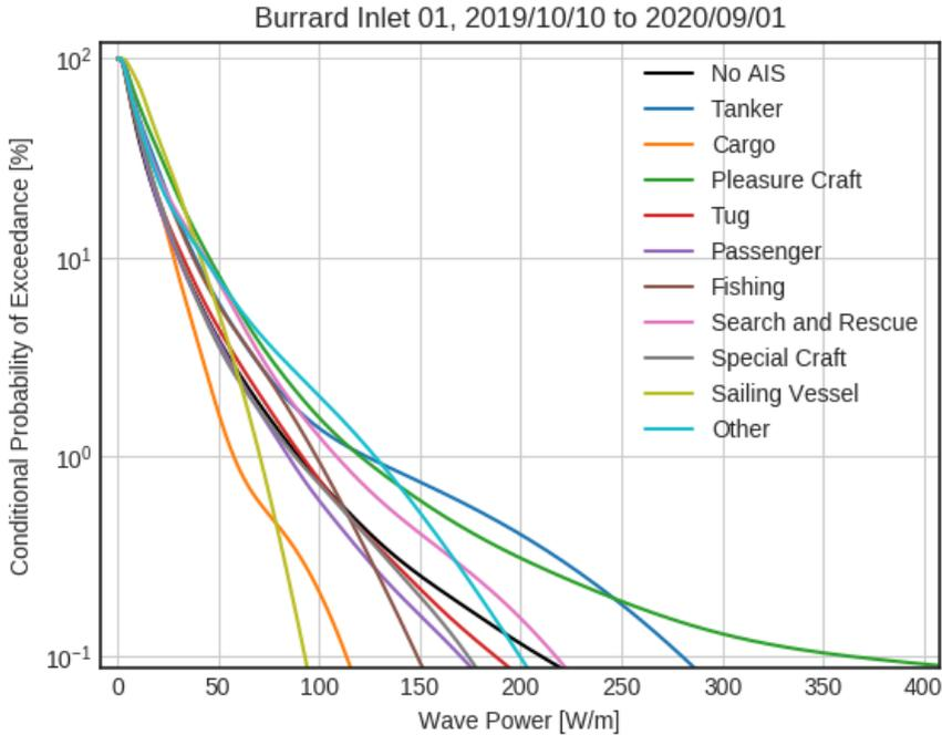
Figure 14: Burrard 1 conditional probability of exceedance distributions based on AIS vessel type.
