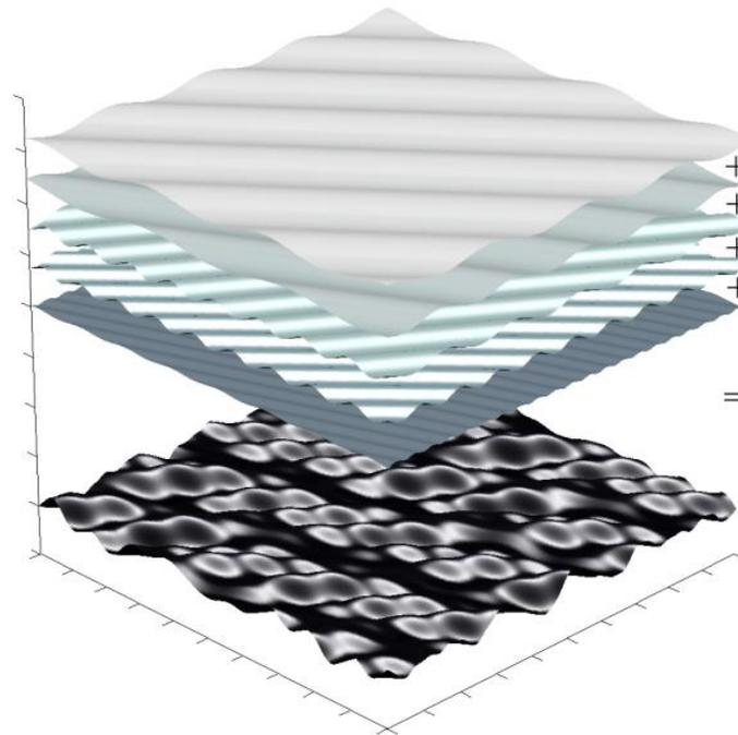
*Figure 3. An illustration of the superposition of ocean waves. Monochromatic propagating waves, shown by the lightly shaded stacked surfaces, of different amplitudes, frequencies, and directions can be superposed to represent the ocean surface shown as the heavily shaded bottom surface.*
