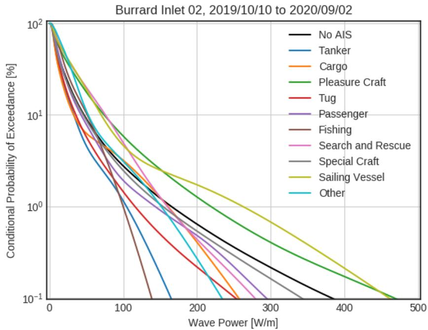
Figure 15: Burrard 1 conditional probability of exceedance distributions based on AIS vessel type.
