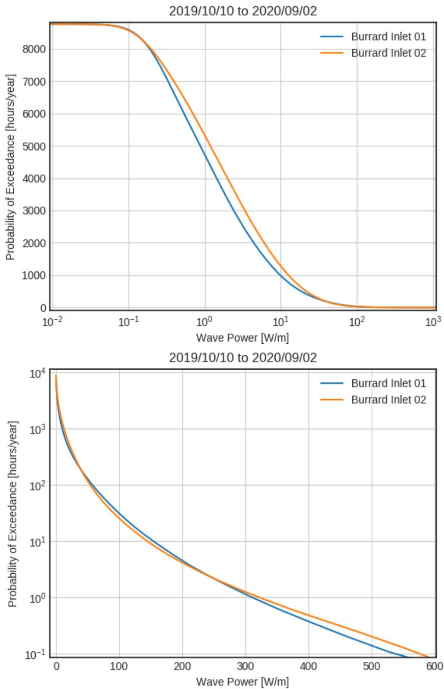
Figure 6: Wave power probability of exceedance for Burrard 1 and 2 buoys. Top: wave power axis is logarithmic. Bottom: probability of exceedance axis is logarithmic
