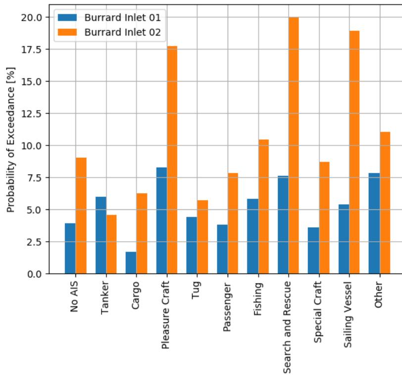
Figure 16: Conditional probability of wave power exceeding 50 W/m for vessel wakes at Burrard 1 and 2.
