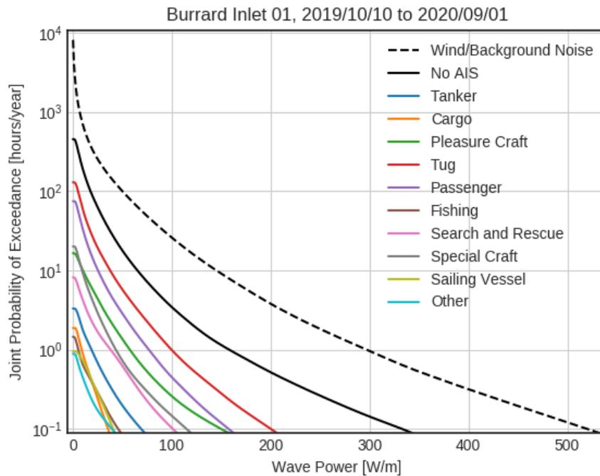
Figure 12: Burrard 1 wave power probability of exceedance distributions based on AIS vessel type.
